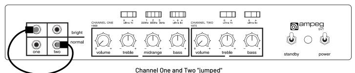
Note: Start with both channel Volume knobs at 0 to avoid loud bursts of audio.
